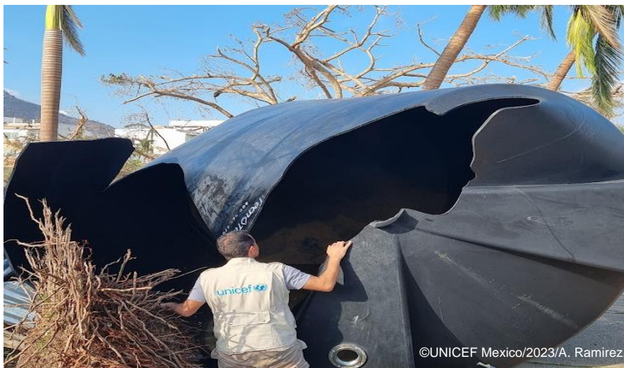
Photo: UNICEF staff assessing damage to a drinking water storage system in Acapulco, Zona Diamante. Reporting period: 1-7 November 2023
